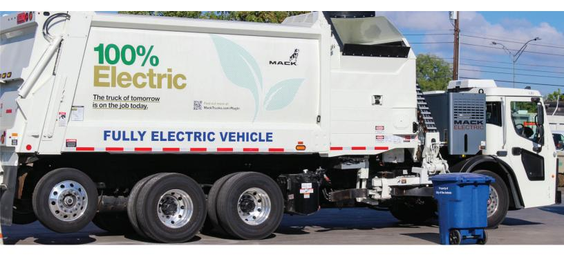
The Department scheduled demos of two different electric garbage trucks in 2022. The first was a Mack LRE chassis with a Heil body. It started off at a VIA Transit Center where the required 480-volt plug was located. Beginning at an 8% charge, the truck took 14 hours to fully charge. The truck picked up roughly 240 carts, made two trips to the landfill and dumped about two tons of material.
